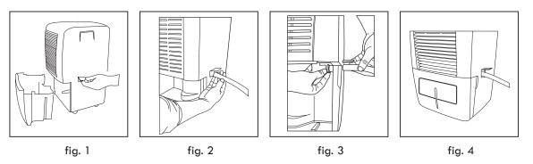
NOTE: If the unit stops operating, check if the bucket full light is illuminated. If it is, remove the bucket, and empty the contents and then check the seal between the hose and the drip tray. If there is a small leak, then replace the hose gasket and re-tighten the hose.
